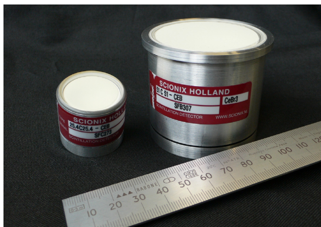
Fig. 1. Picture of two of the CeBr 3 encapsulated samples used in this study, left 1" × 1" sample SFC 273 (proton irradiated) and right 2" × 2" sample SFB 307.
